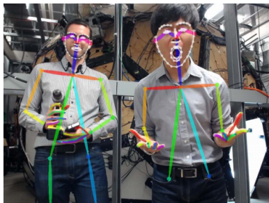
Figure 14.32: Illustration of keypoint detection for body, hands and face using the OpenPose system. From Figure 8 of [Cao+18]. Used with kind permission of Yaser Sheikh.
