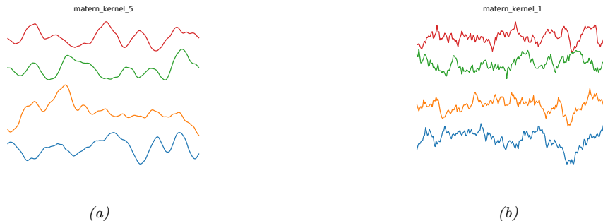
Figure 17.2: Functions sampled from a GP with a Matern kernel. (a) \nu = 5/2 . (b) \nu = 1/2 . Generated by gpKernelPlot.ipynb .
