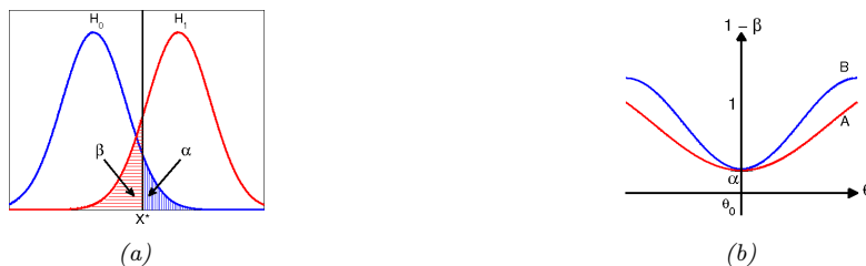
Figure 5.10: (a) Illustration of the Neyman-Pearson hypothesis testing paradigm. Generated by neyman-Pearson2.ipynb . (b) Two hypothetical two-sided power curves. B dominates A. Adapted from Figure 6.3.5 of [LM86]. Generated by twoPowerCurves.ipynb .
