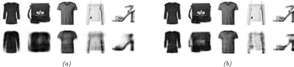
Figure 20.17: Results of applying an autoencoder to the Fashion MNIST data. Top row are first 5 images from validation set. Bottom row are reconstructions. (a) MLP model (trained for 20 epochs). The encoder is an MLP with architecture 784-100-30. The decoder is the mirror image of this. (b) CNN model (trained for 5 epochs). The encoder is a CNN model with architecture Conv2D(16, 3 × 3, same, selu), MaxPool2D(2 × 2), Conv2D(32, 3 × 3, same, selu), MaxPool2D(2 × 2), Conv2D(64, 3 × 3, same, selu), MaxPool2D(2 × 2). The decoder is the mirror image of this, using transposed convolution and without the max pooling layers. Adapted from Figure 17.4 of [Gér19]. Generated by ae_mnist_tf.ipynb .
